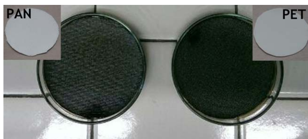
Figure 1. PAN (on the left) and PET (on the right) fabrics coated with PDA (in the inset, the pristine PAN and PET fabrics). [Color figure can be viewed in the online issue, which is available at wileyonlinelibrary.com .]
